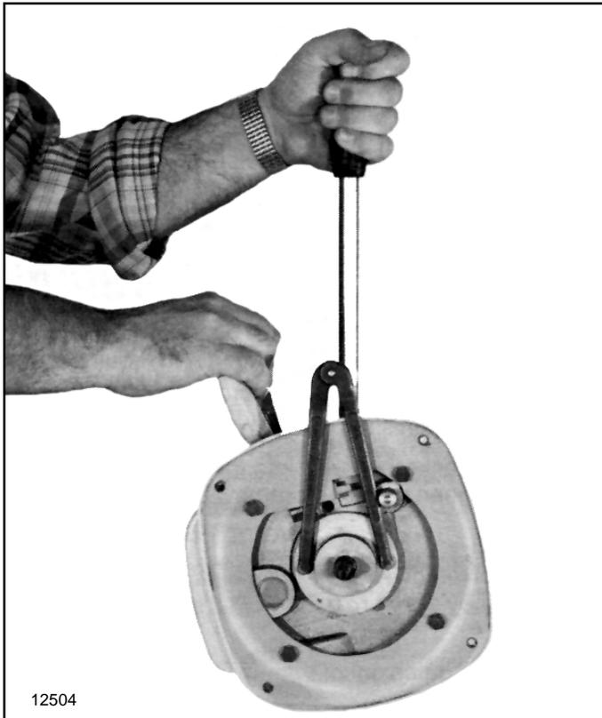
**Figure 7-2. Removing Load Brake Flange**
