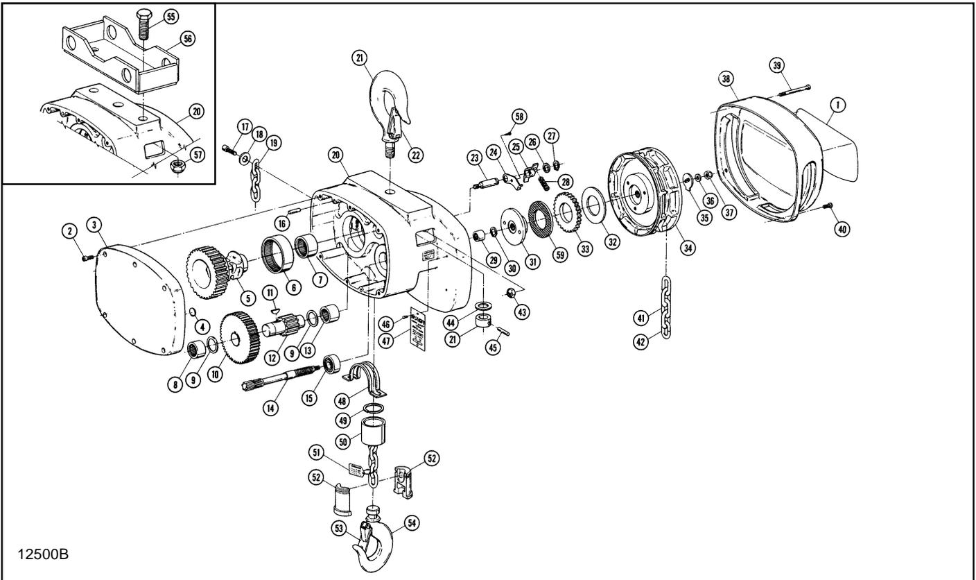
Figure 9-3. 1½ and Single Load Chain 2 Ton Models
