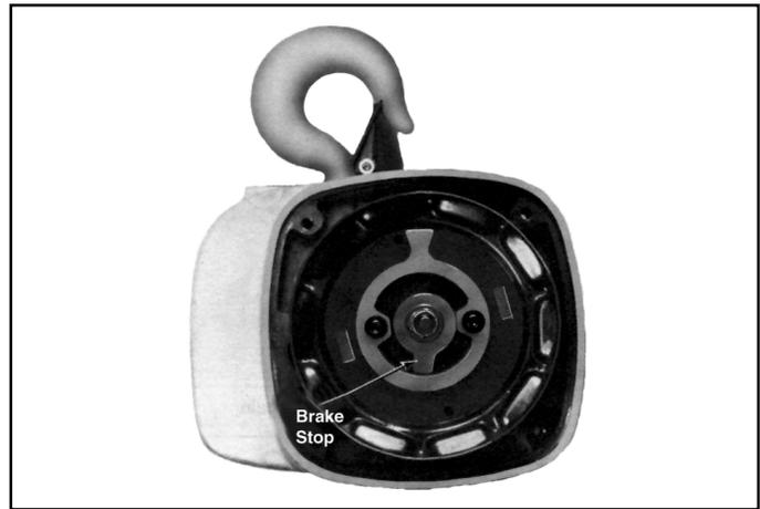
**Figure 7-6. Brake Stop Position for 1/4 and 1/2 Ton Models**
